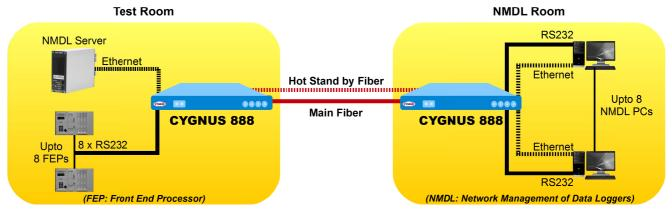
A CYGNUS 888 pair used to extend up to 8 RS232 ports of FEPs from Test Room to NMDL Room. Simultaneously the processed data from the NMDL PCs is send back to NMDL Server using Ethernet port
