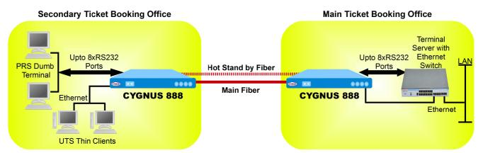
A CYGNUS 888 pair used to extend up to 8 RS232 Dumb Terminals and Ethernet Thin Clients from the main Booking Office at a station to a secondary Booking Office there
