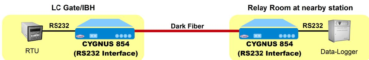
Connecting RTU at a LC Gate/IBH to Data Logger in the Relay Room of a nearby station, using Dark Fiber
