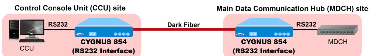
Connecting CCU at a station to MDCH using Dark Fiber
