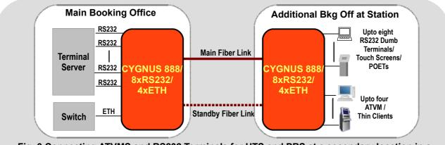
Fig. 3 Connecting ATVMS and RS232 Terminals for UTS and PRS at a secondary location in a railway station using a pair of CYGNUS 888 Fiber Optic Multiplexers connected over Fiber
