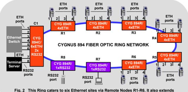
Fig. 2 This Ring caters to six Ethernet sites via Remote Nodes R1-R6. It also extends two RS232 ports of a central Terminal Server through Remote Nodes R7 and R8 which have 1 RS232 port each.
