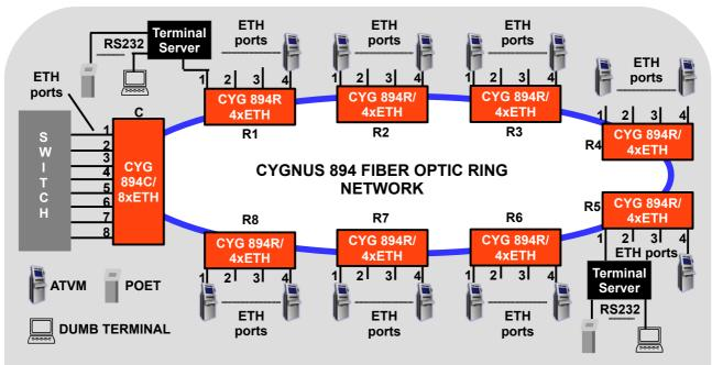
Fig. 1. Distributing ATVMs and Terminal Servers at various places in a station premises on a fiber optic ring. CYGNUS 894C Central Node (C) is used for access to upstream Switch. CYGNUS 894R Remote Nodes (R1-R8) are located at the ATVM / Terminal Server sites.
