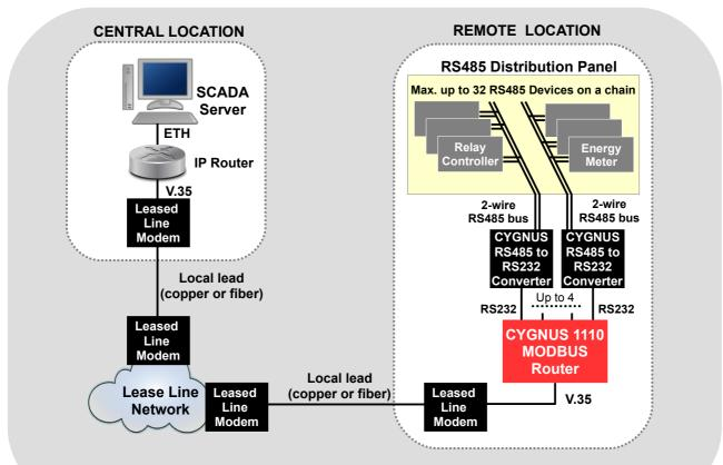
Fig. 2. CYGNUS 1110 Modbus Router connected to a centrally located SCADA Server connected over a leased WAN Link of 64k/2Mbps capacity.
