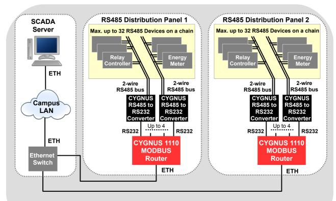
Fig. 1. CYGNUS 1110 Modbus Routers used to access data from Energy Meters
